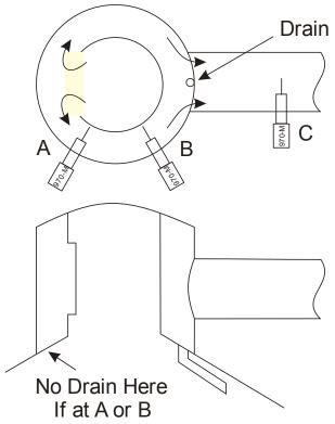
DOWNSCALE ERRORS are generally caused by water addition to the vapor stream before it reaches the vapor bulb. Even small quantities of water can appreciably desuperheat the vapor and destroy monitor accuracy and reliability. Here are some of the places where this can occur, with suggestive corrective measures:
