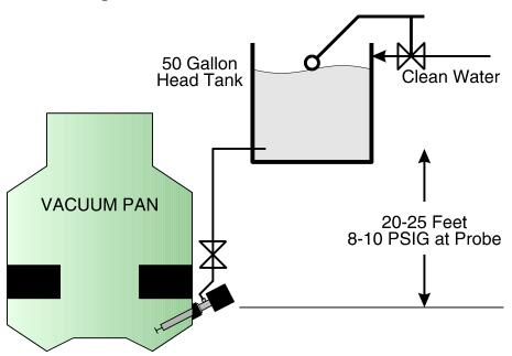
Figure 3: 971-C Head Tank Location
