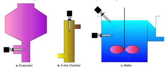
Figure 2: Probe Mounting Configurations
