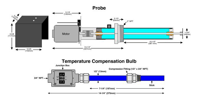
Figure 1: Mounting Dimensions for Sensor
