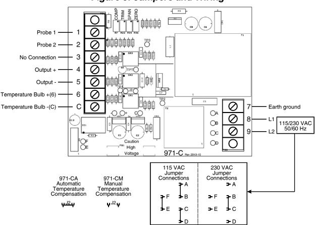
Figure 5: Jumpers and Wiring
